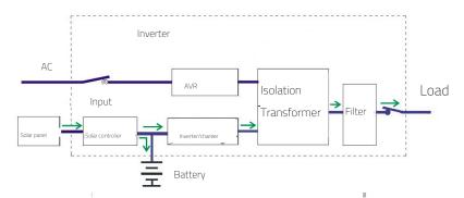
If solar energy less than output power, the system will convert the energy of battery and PV systems and give power supply to the user equipment.
