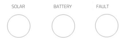
Left : Green LED: Solar panel connect state. Long light means normal. Light off or flash means connect unusualMiddle Yellow LED: Battery connect state : long light means normal, light off or flash means connect unusualRight Red Led : means abnormal state, light means solar part abnormal
