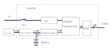
During the evening (or rainy days, with no sun), the system will convert the energy of battery and give power supply to the user equipment.
