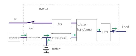
If battery capacity less than 30%, the inverter turn off and no power supply to de user equipment. At this time, solar energy can charge the battery normally.
