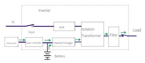
If battery capacity less than 40%, AC input will provide power to equipments through regulator by relays and transformer. At this time, PV gives power to batteries only through MPPT control system.
