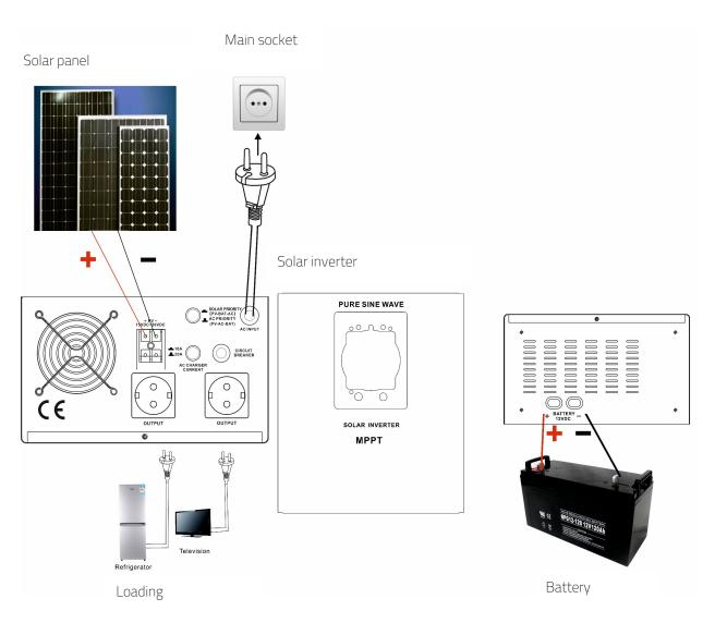
Connection diagram (3KVA to 5KVA)
