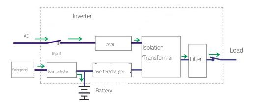
During the evening (or rainy days, with no sun), AC power will charge battery by charger inside the inverter.
